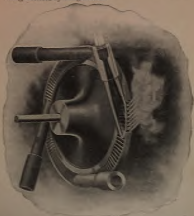
FIG. 12.—Runner and Nozzle of De Laval Steam-turbine. Built by the De Laval Steam Turbine Co., Trenton, N. J.
